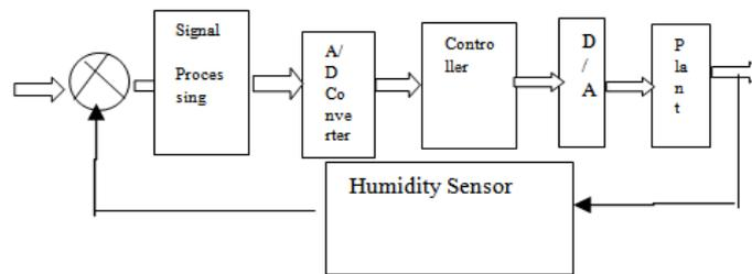
**Figure 4: Operation of Humidity Sensor.**
