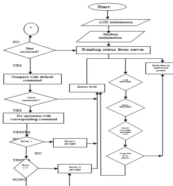
Figure 7: Flow Diagram of Micro Controller.
