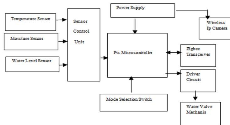
**Figure 1: Sensor Control Unit.**
